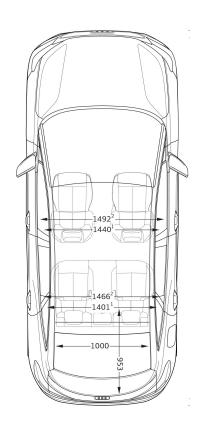
Q4 Sportback e-tron - luggage compartment capacity: 535l (rear seats up) or 1460l (loaded up to roof with rear seats folded).
