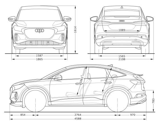
Dimensions in millimetres. Optional equipment may affect dimensions. Dimensions were measured with vehicle at unladen weight, ground clearance measured with vehicle carrying its maximum load. Turning circle approx.10,200mm.
