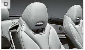
Exclusively available for BMW M4 Convertible Competition, the air collar releases pleasant, warm air around the head and shoulders, ensuring comfort when driving with the roof open.
